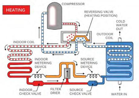
Heat pumps squeeze warmth out of cold air
